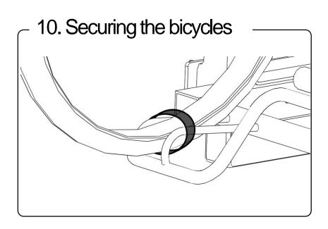
Now the bicycles can be further secured around the wheels by means of the lashing straps included. The bicycle, or bicycles, are now fully secured onto the Tilly Light.
