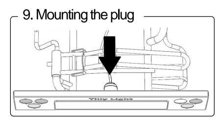
Mount the light plug to the back of the light bar. First, place the plug into the light bar. Turn it a quarter turn until the plug is firmly connected.
