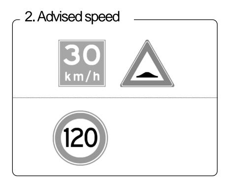
The advised speed when crossing a speed ramp with the Tilly Light is 30 kilometres per hour.
