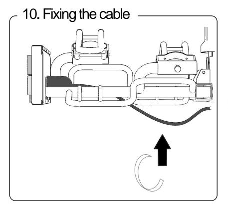
Connect the plug cable to the bicycle carrier and secure it by means of the Velcro strips, so that it will not drag along the ground.
