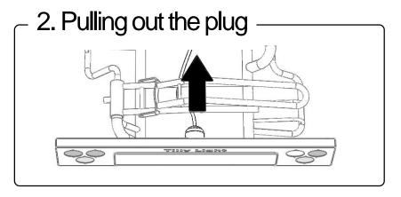
Remove the light plug from the light bar by turning it a quarter turn and pulling out the plug.
