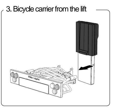
Take the bicycle carrier from the lift by slightly tilting the light bar while lifting the bicycle carrier.
