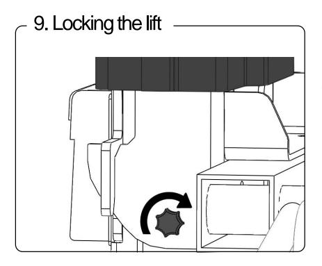
Lock the lift using the lock bolt on the right-hand side of the lift by fully tightening it.
