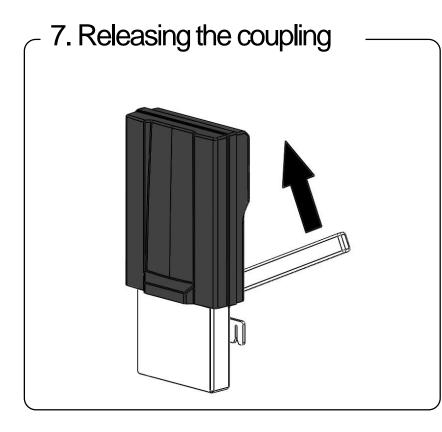
The tow-hook coupling is released by moving the lever up.
