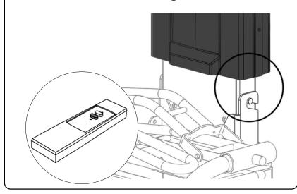
Position the lift at the correct height by ensuring that both the suspension stud and the suspension hook are fully visible.
