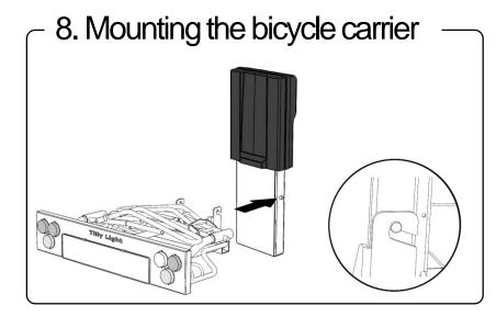
Mount the bicycle carrier onto the lift in such a way that the suspension hook of the bicycle carrier falls around the suspension stud of the lift.
