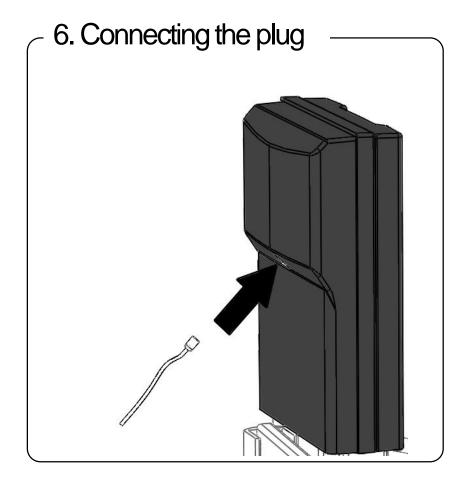
Connect the female plug to the plug at the back of the lift. Secure it using the lock on the contact plug.
