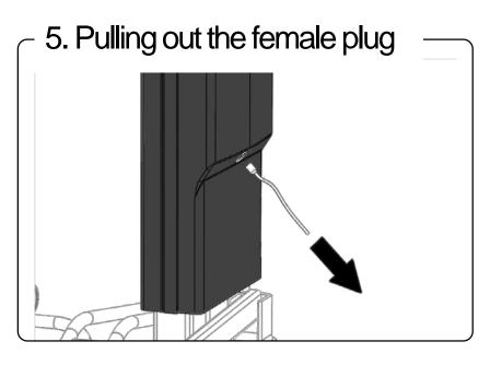
Unlock the contact plug by tipping up the lock. Next, remove the female plug from the lift.
