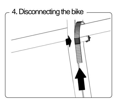
Release the bike by pressing in the buckle and opening the ratchet strap.
