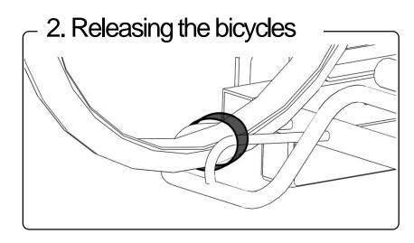
Loosen the straps around the wheels. Next, mount the straps onto the Tilly Light so that they are at hand when you next use the bicycle carrier.
