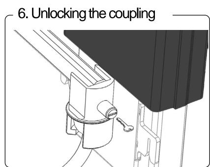
Use the key to unlock the towing-hook coupling.
