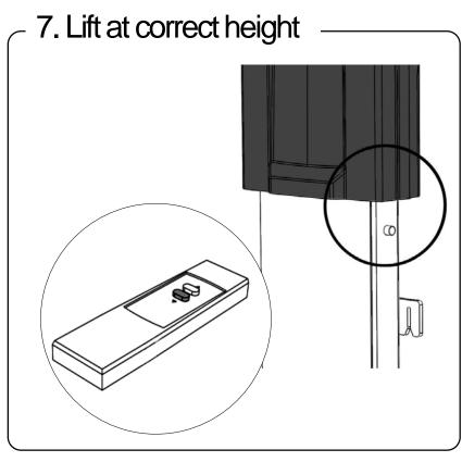
Position the lift at the correct height by ensuring that the suspension stud is at least 4 centimetres underneath the protective cover.
