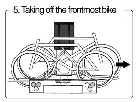
Ride the frontmost bike backward off the bicycle carrier. The front-wheel support will follow the movement.
