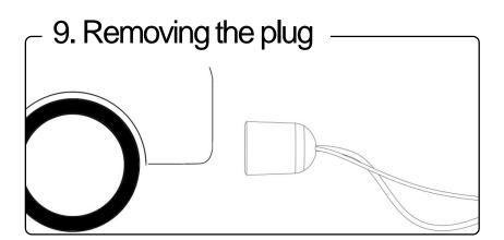
Disconnect the car's plug by turning it a quarter turn and pulling it out.
