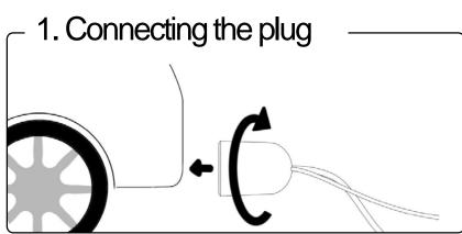
Start by connecting the car plug. First, place the plug in the car's socket. Turn it a quarter turn until the plug is firmly connected.
