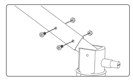
Position the bolts in the holes in the lever. Tighten the nuts to the bolts on the other side of the lever. Use the spanner and screwdriver.
