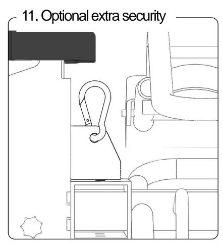
The carabine hook on the bicycle carrier offers the possibility to mount extra straps for securing the bicycles.
