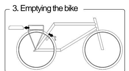
• Make sure that all loose parts, such as the battery and the bicycle computer, are removed from the bike before transporting it.
