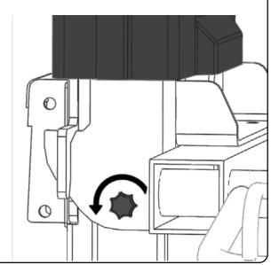
Loosen the lock bolt to unlock the lift.
