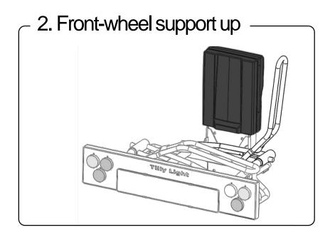
Move the rearmost frontwheel support up as shown in the drawing.
