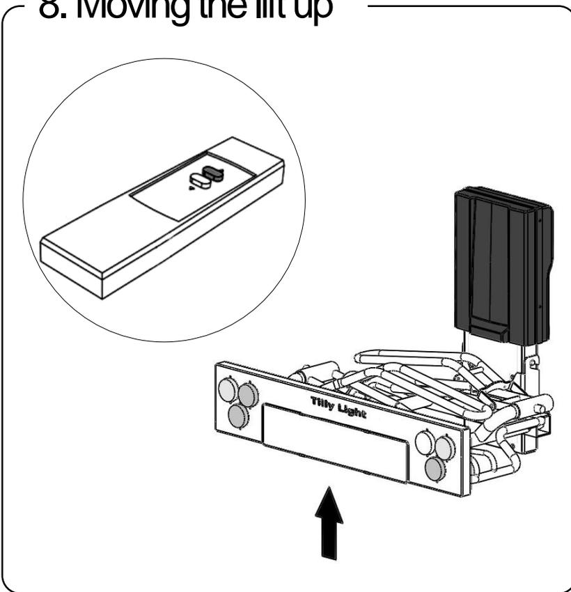
Move the lift up using the remote control.
