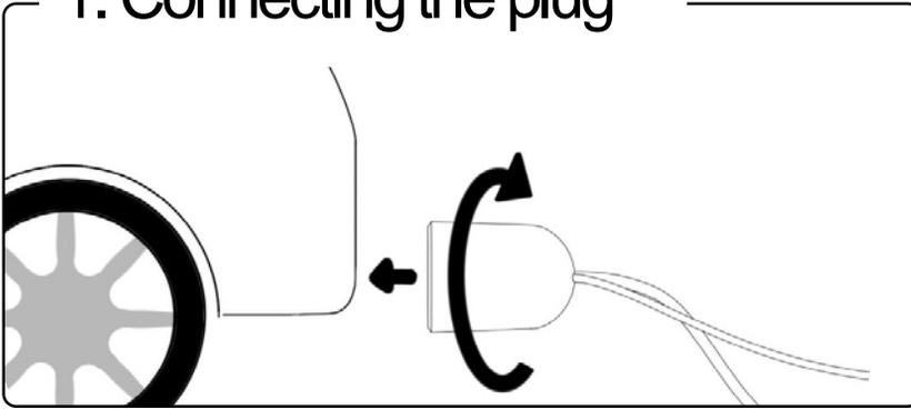
Start by connecting the car plug. First, place the plug in the car's socket. Turn it a quarter turn until the plug is firmly connected.
