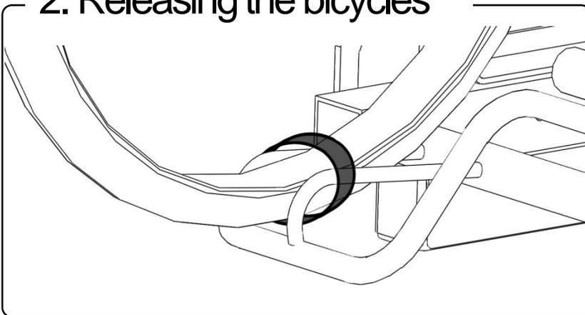
Loosen the straps around the wheels. Next, mount the straps onto the Tilly Light so that they are at hand when you next use the bicycle carrier.
