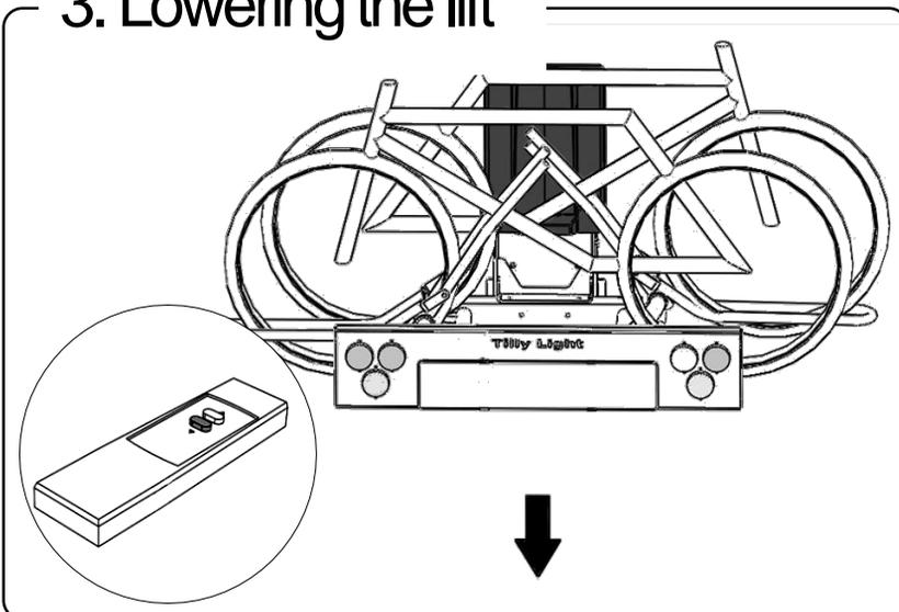
Lower the lift using the remote control.
