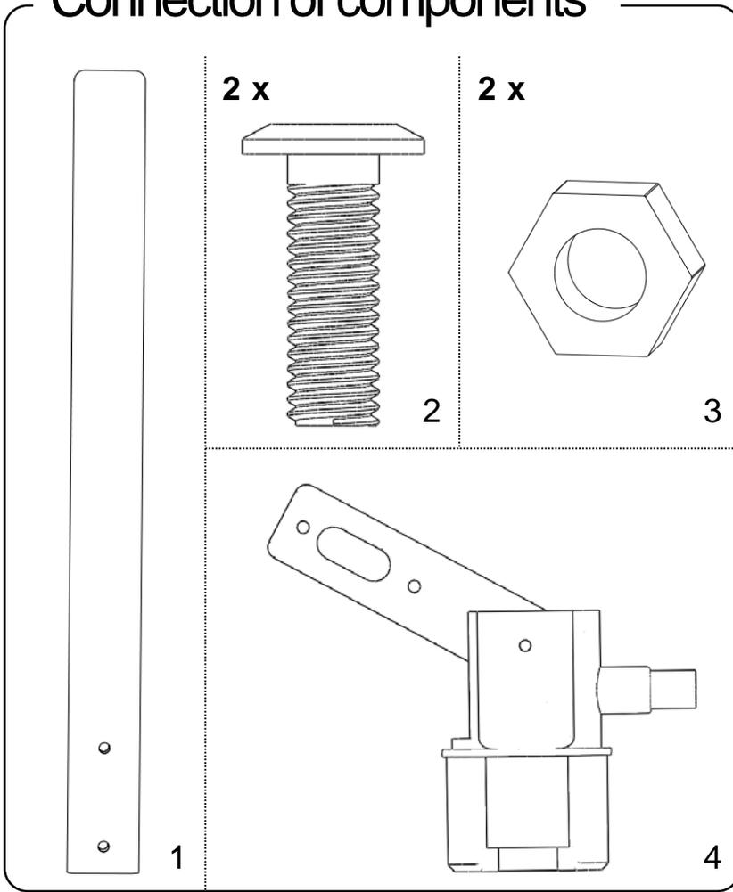
Before installing the Tilly Light, the lever must be mounted to the towing-hook coupling. The lever (1) is mounted to the towing-hook coupling by means of 2 bolts (2) and 2 nuts (3).
