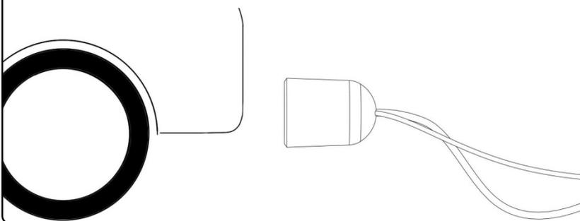
Disconnect the car's plug by turning it a quarter turn and pulling it out.
