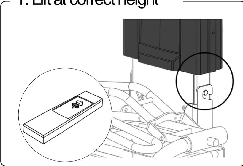
Position the lift at the correct height by ensuring that both the suspension stud and the suspension hook are fully visible.
