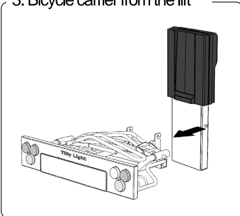
Take the bicycle carrier from the lift by slightly tilting the light bar while lifting the bicycle carrier.
