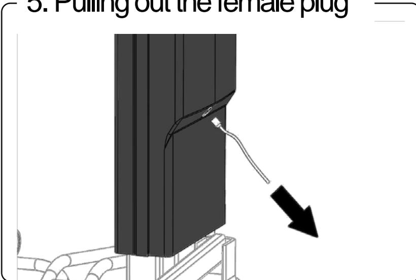
Unlock the contact plug by tipping up the lock. Next, remove the female plug from the lift.
