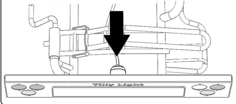
Mount the light plug to the back of the light bar. First, place the plug into the light bar. Turn it a quarter turn until the plug is firmly connected.
