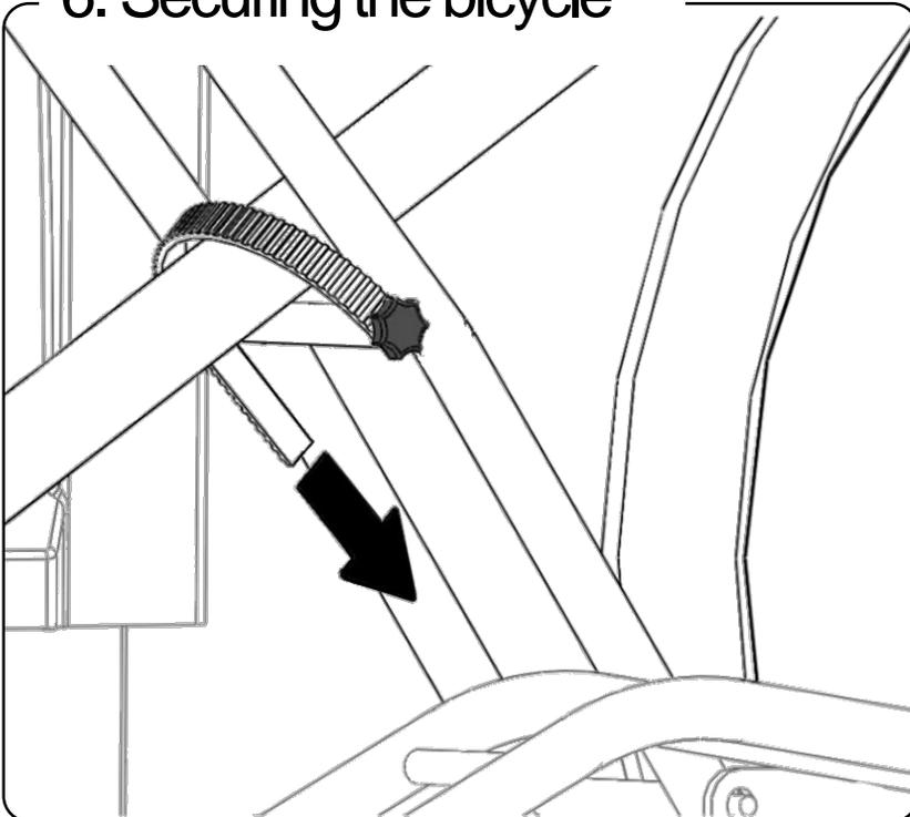
Lock the bicycle and secure it using the ratchet strap.
