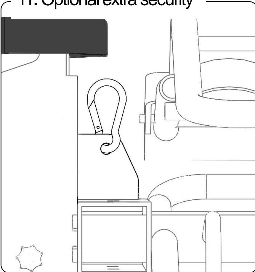
The carabine hook on the bicycle carrier offers the possibility to mount extra straps for securing the bicycles.
