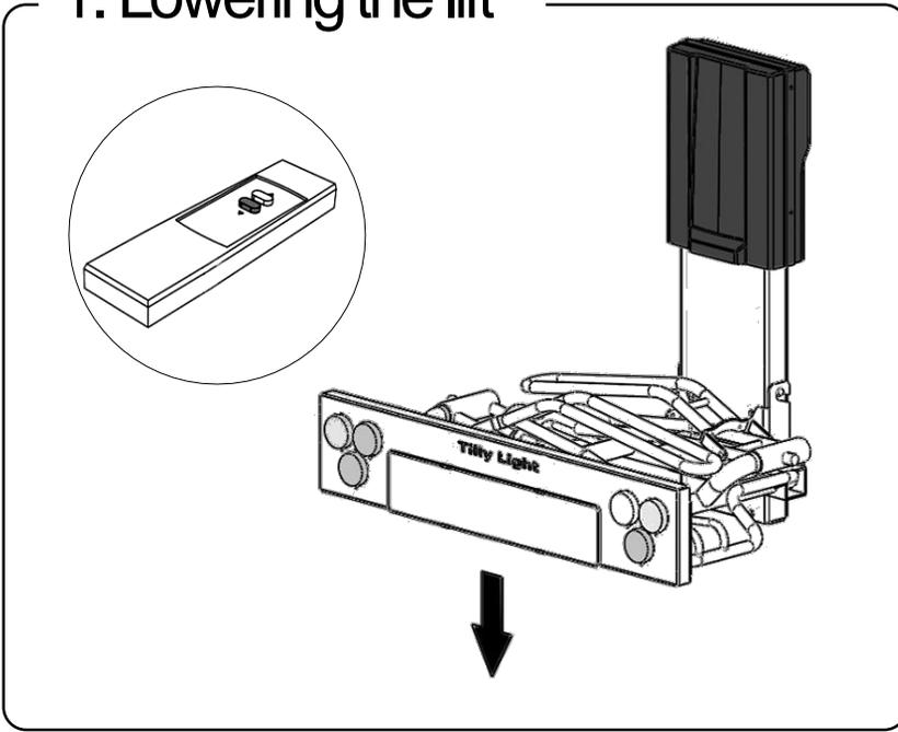
Lower the lift to its lowermost position using the remote control.
