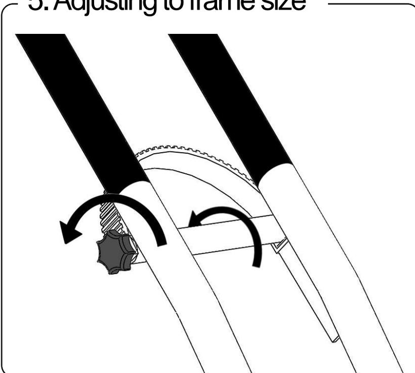
The height of the front-wheel support tube can be adjusted. By loosening the star bolt and the tube, the front-wheel support tube can be slid up and down.
