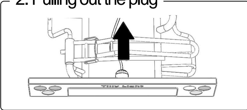
Remove the light plug from the light bar by turning it a quarter turn and pulling out the plug.
