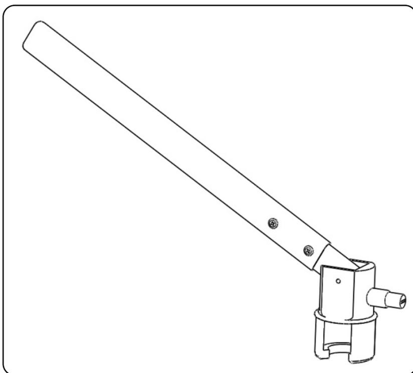
Make sure the lever is well connected to the towing-hook coupling. The lever must be connected to the towing-hook coupling as shown in the drawing.
