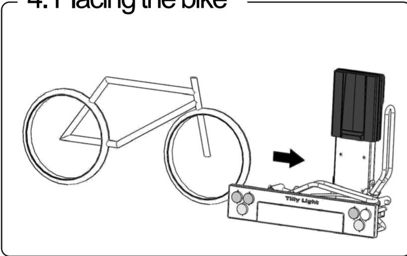
Ride the bicycle into the rearmost front-wheel support from the side. Make sure the left-hand pedal points to the rear of the bicycle.
