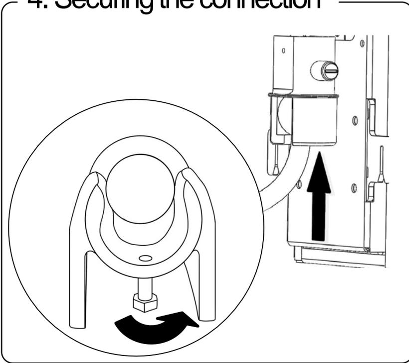
At the bottom of the towing-hook coupling is a bolt that should touch the towing hook. Should it not touch the towing hook, tighten it until it does.
