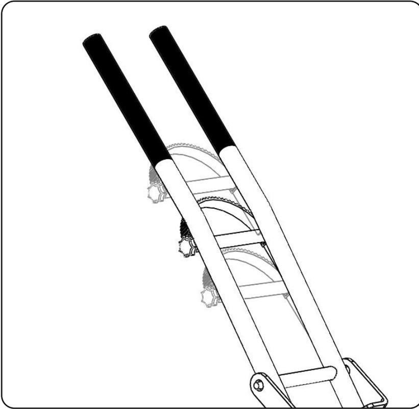
Slide the front-wheel support tube to the desired height. Slide it up if there is play between the frame and the tube. Slide it down if it is not possible to ride the bicycle completely onto the front-wheel support.
