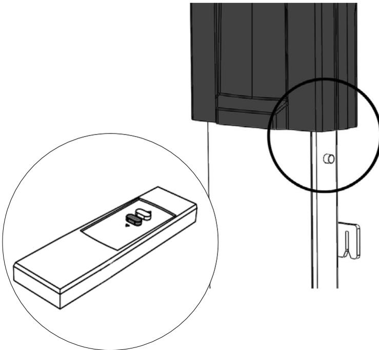
Position the lift at the correct height by ensuring that the suspension stud is at least 4 centimetres underneath the protective cover.
