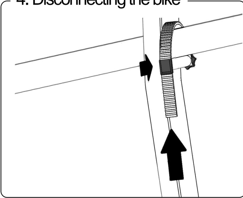
Release the bike by pressing in the buckle and opening the ratchet strap.
