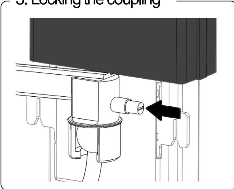
Secure the towing-hook coupling by pushing in the lock.
