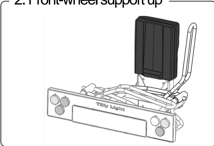
Move the rearmost front-wheel support up as shown in the drawing.
