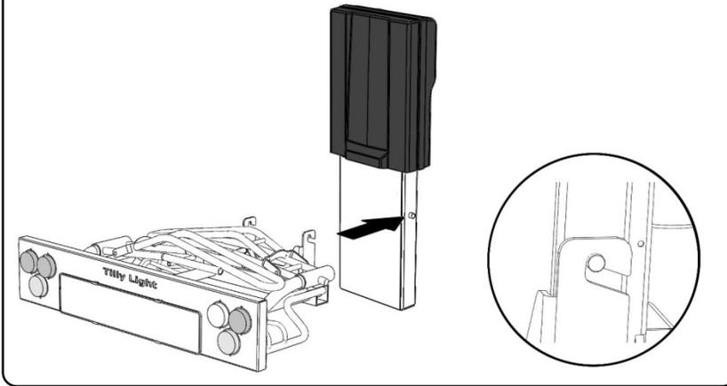
Mount the bicycle carrier onto the lift in such a way that the suspension hook of the bicycle carrier falls around the suspension stud of the lift.
