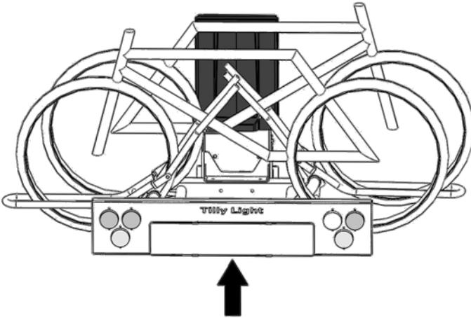
Move the lift up to its uppermost position using the remote control.
