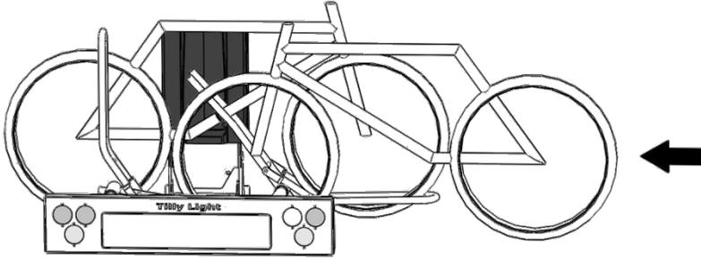
Move the frontmost bicycle clamp up and ride the second bike onto the front-wheel support in the opposite direction. Make sure the left-hand pedal points to the front of the bicycle. Secure this bicycle by means of the ratchet strap as well.
