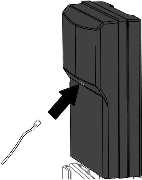
Connect the female plug to the plug at the back of the lift. Secure it using the lock on the contact plug.
