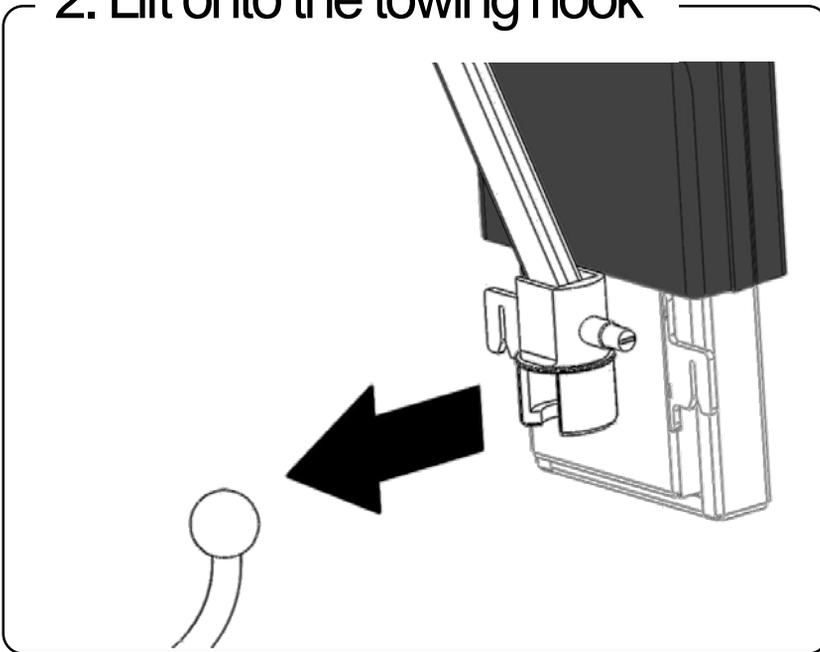
Place the lift onto the car's towing hook by placing the ball into the lift's towing-hook coupling.
