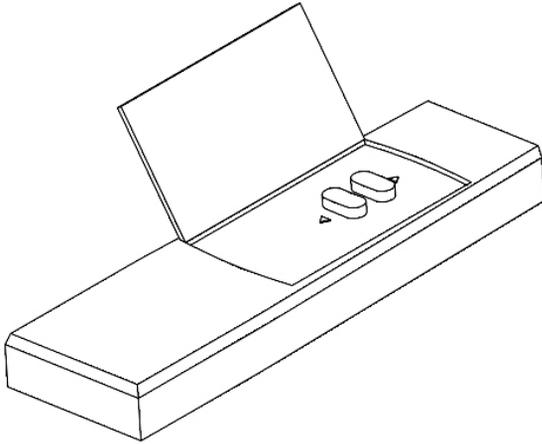
Fold down the lid of the remote control. Make sure the remote control is stored in a safe place in the car, so that it cannot be operated accidentally as a result of the car's movements causing the lift to be activated while driving.
