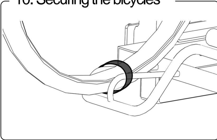
Now the bicycles can be further secured around the wheels by means of the lashing straps included. The bicycle, or bicycles, are now fully secured onto the Tilly Light.
