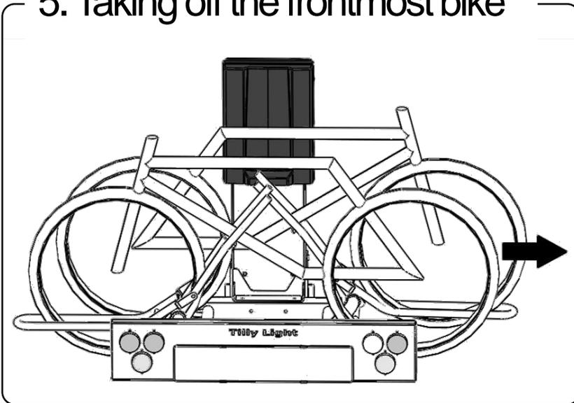
Ride the frontmost bike backward off the bicycle carrier. The front-wheel support will follow the movement.
