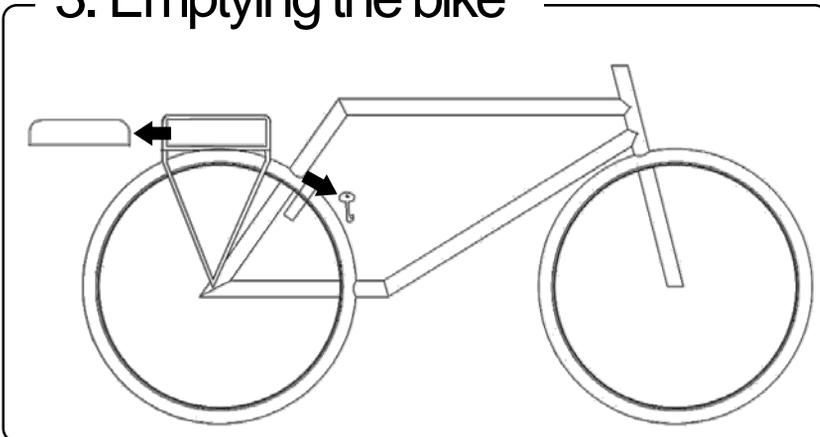
**!** Make sure that all loose parts, such as the battery and the bicycle computer, are removed from the bike before transporting it.
