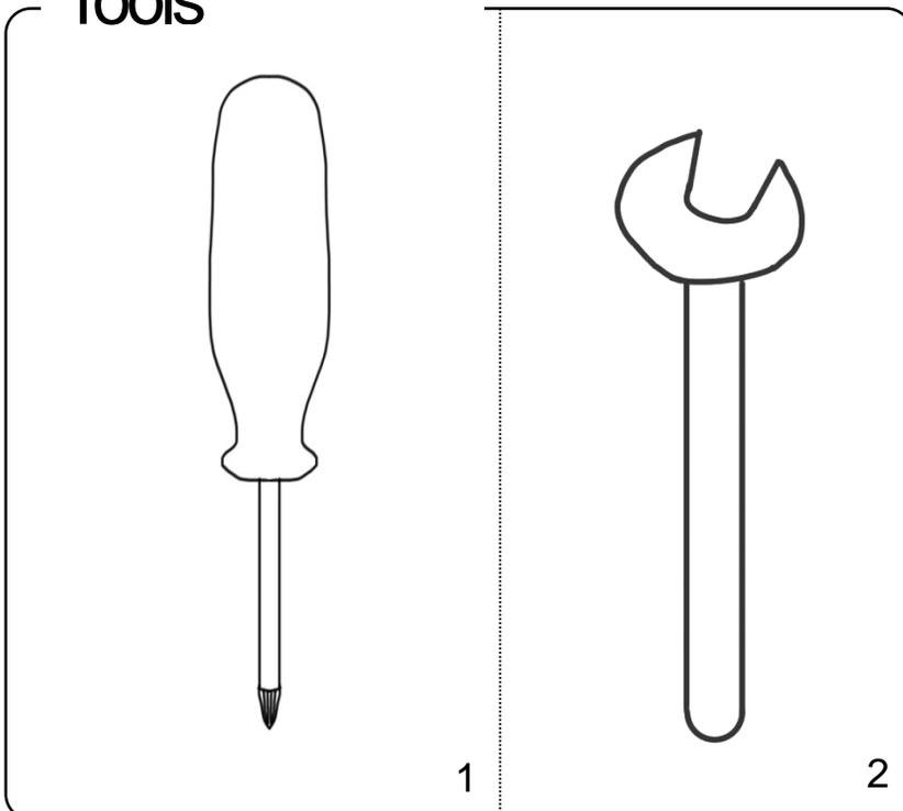
The lever is mounted using a crosshead screwdriver (1) and a spanner size 10 (2).
