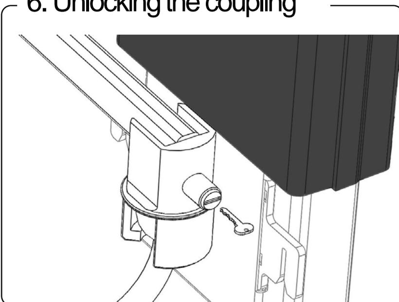
Use the key to unlock the towing-hook coupling.
