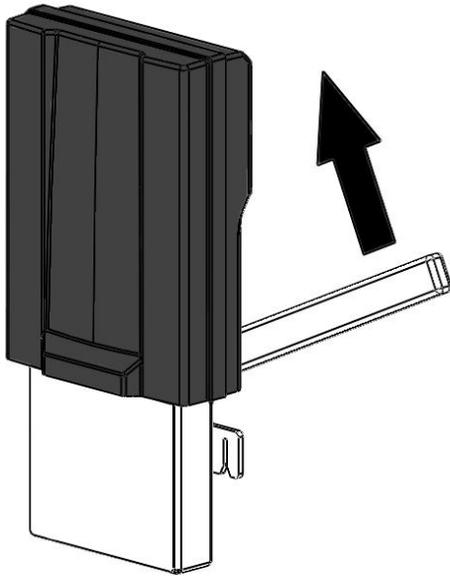
The tow-hook coupling is released by moving the lever up.
