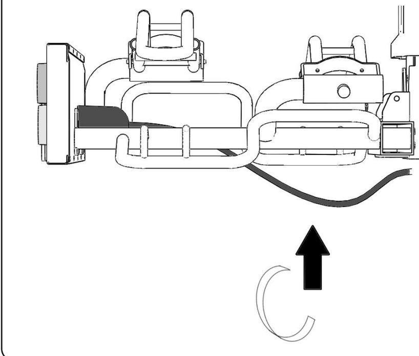
Connect the plug cable to the bicycle carrier and secure it by means of the Velcro strips, so that it will not drag along the ground.
