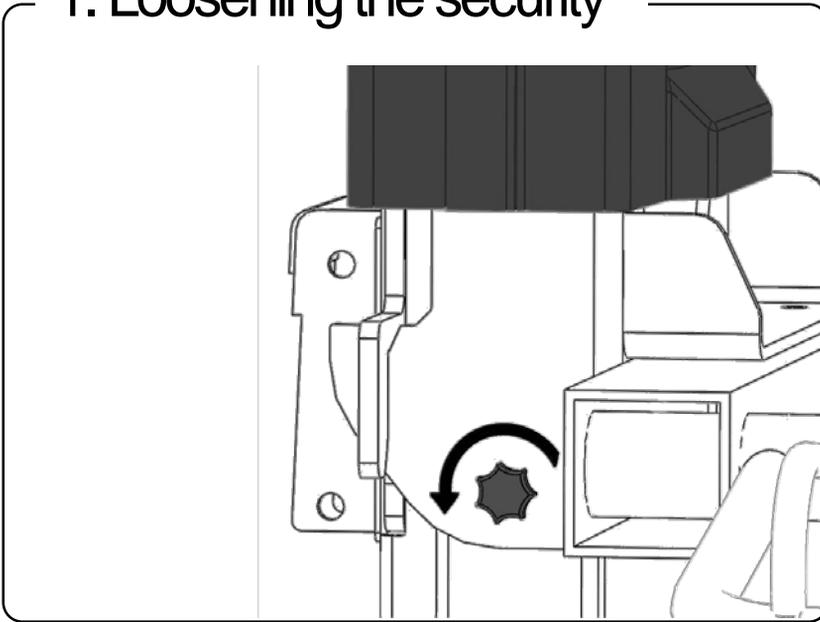
Loosen the lock bolt to unlock the lift.
